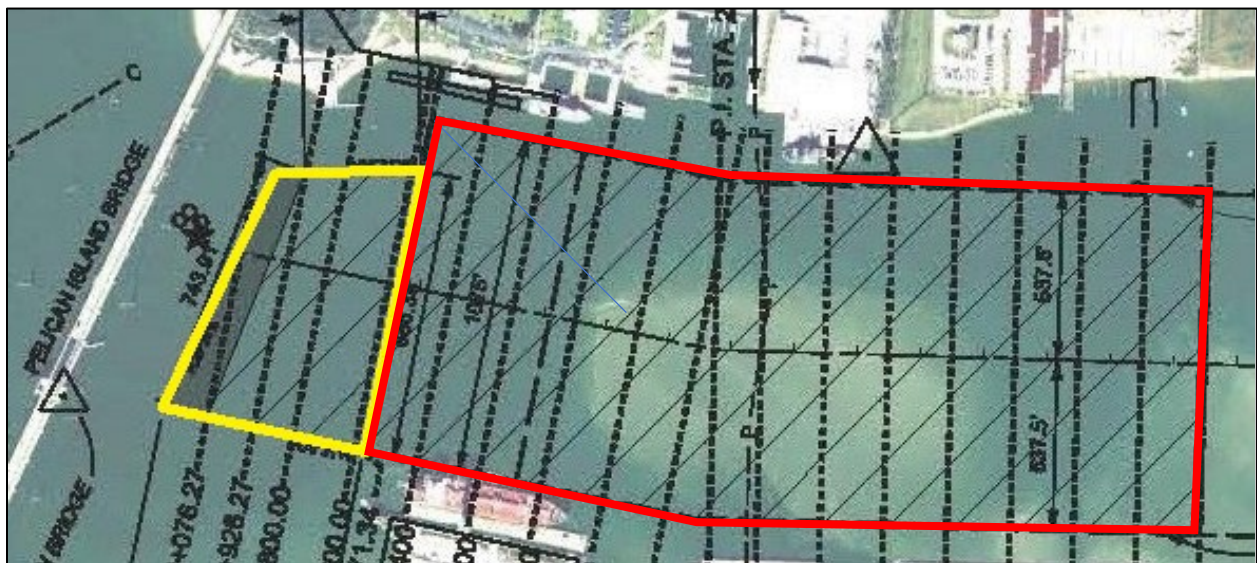
Figure 2 - Aerial Drawing of Authorized Project (red) Showing Increase in Footprint for Addition of Channel Extension (yellow)
